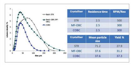
The results have been demonstrated on both model compounds and products of true industrial interest and have shown a significant improvement in yield and ability to control PSD. The complete COBR with PAT enhanced automation is currently being demonstrated at the Centre for Innovative Manufacturing and Crystallisation at the University of Strathclyde.
